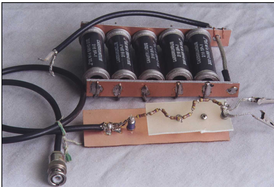
Fig 12—Two devices that help to test the diplexer filters. At the top is a 150-W dummy load that is mentioned in the text. At the bottom is a high-impedance probe for testing the LPF and HPF filter outputs.
